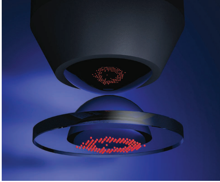
Figure 1.1: Concept of the quantum gas microscope. A degenerate gas of ultracold atoms resides in a two-dimensional lattice, a few microns away from the final lens of a high resolution imaging system. The lattice spacing is small enough ( \approx 0.5\mu m ) to achieve a strongly correlated quantum gas which can be used to simulate the physics of condensed matter systems. The high resolution system allows the imaging and addressing of individual atoms in the lattice, capabilities similar to those provided by scanning tunneling microscopy of solids.
